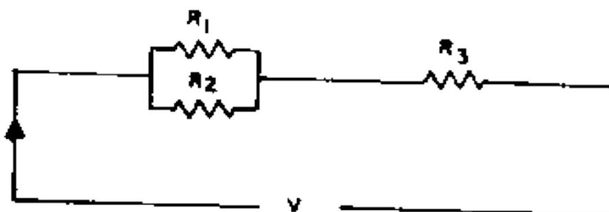
$$\begin{aligned}R_1 &= 6 \Omega \\R_2 &= 4 \Omega \\R_3 &= 3,6 \Omega\end{aligned}$$
