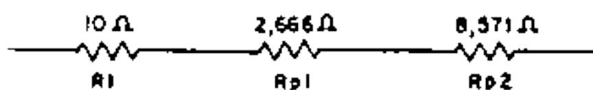
$$R_t = R_1 + R_{p1} + R_{p2} = 10 + 2,666 + 8,571 = 21,23\ \Omega \approx 21,2\ \Omega$$
